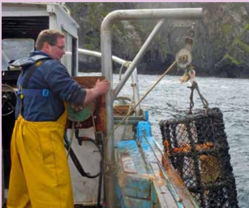
A derrick and snatch block is most commonly used to bring pots on board but some vessels also use a roller to bring the pot over the gunwale and land it onto a stainless steel table.
