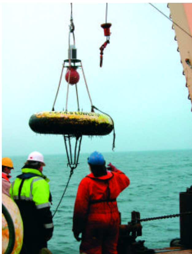
Fig 6.3 Retrieving a wave monitoring buoy. John Costelloe, Aquafact International Services, Ireland.
