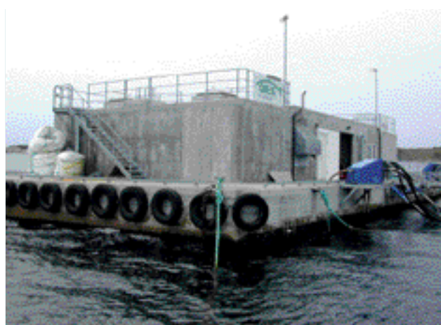
Fig 6.9 Concrete box feed barge. Marine Construction, Norway.
