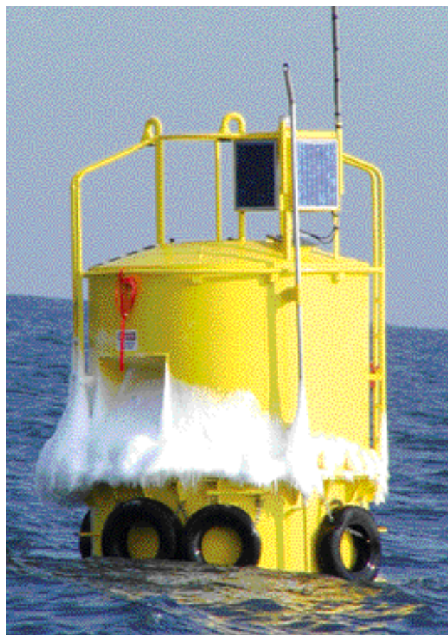
4.21(b) Prototype spar feed buoy for supply of feed to submerged cages off the coast of New Hampshire, USA. University of New Hampshire.
