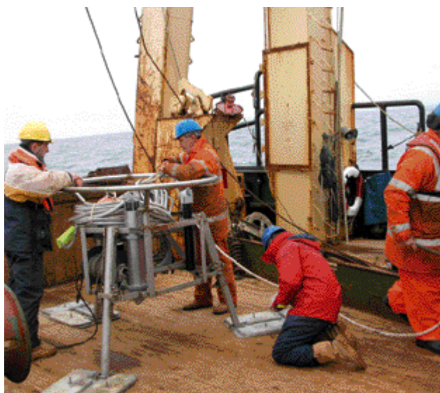
Fig 6.2 Preparing a sea-bed located, current and environment monitoring device for deployment. John Costelloe, Aquafact International Services, Ireland.
