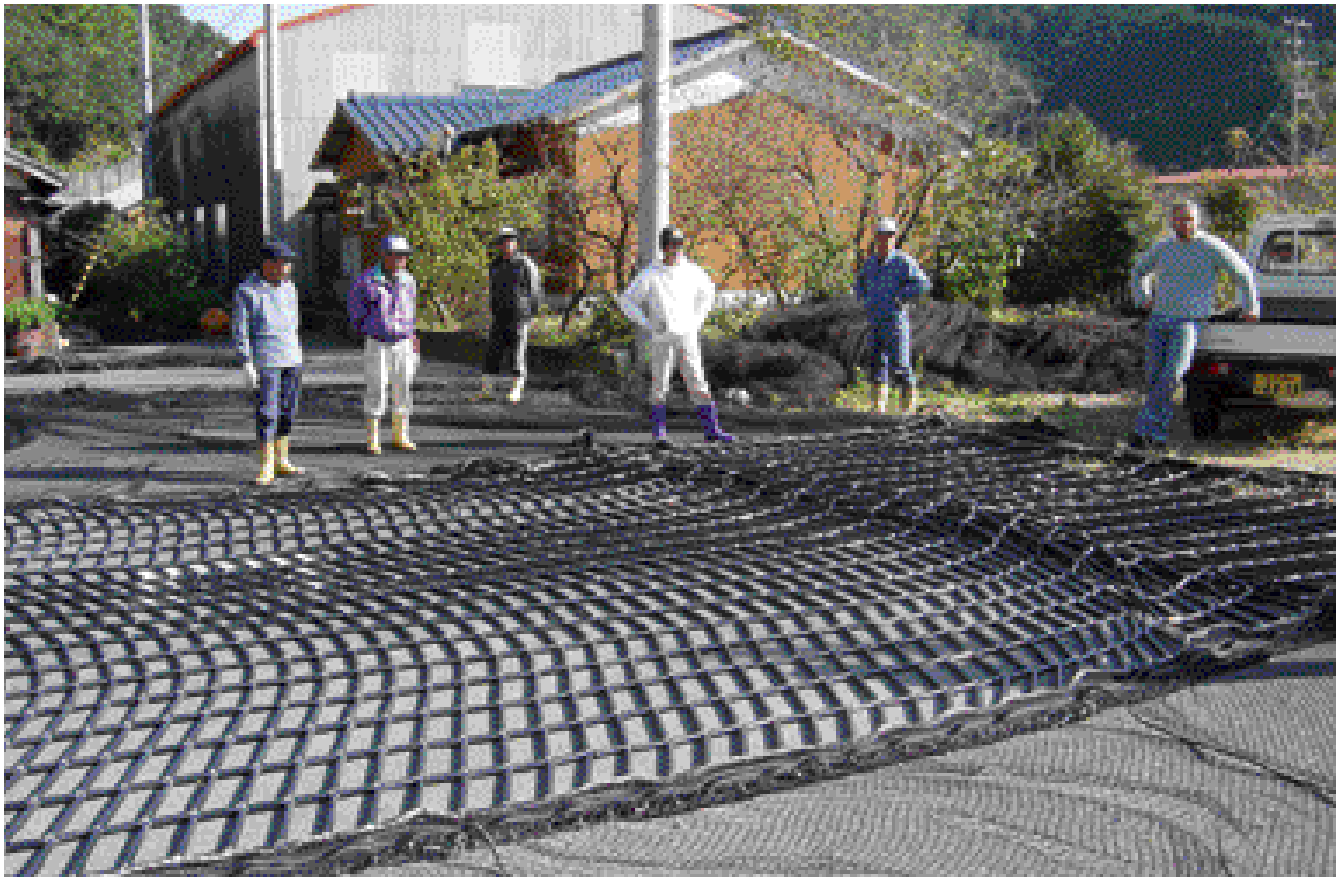
Fig 7.1(a) Fish grading panel sown into seine net. Grading Systems (UK) Ltd.
