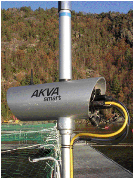
Fig 3.24(b) Data transmission system for submersible camera and doppler system. Akvasmart, Norway.
