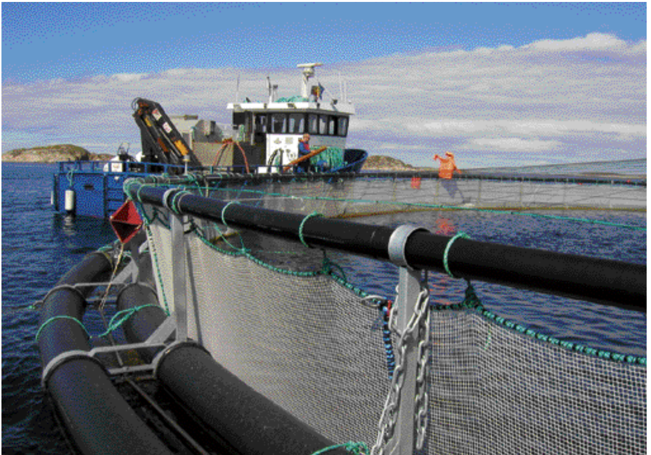
Fig 1.7 Highly specialised work boat with lifting crane and feed cannon feeding a 120-metre circumference plastic collar cage, Norway. Aqualine, Norway.
