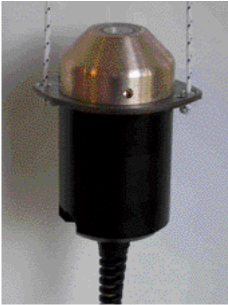
Fig 3.24(a) Submersible camera for monitoring fish appetite and behaviour. Akvasmart, Norway.
