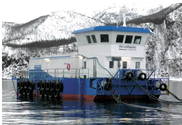
Fig 3.21 Feed barge in steel with high storage capacity. Akvasmart, Norway.
