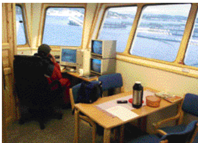
Fig 3.22 Feed barge control system. Note monitors for cameras, appetite, and feed administration. Akvasmart, Norway.
