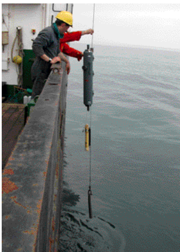
Fig 5.3 Water sampling on a monthly basis is required by Government regulation at Irish fish farm sites. Samples are analysed for temperature, salinity, nutrients, oxygen and chlorophyll. John Costelloe, Aquafact International Services.
