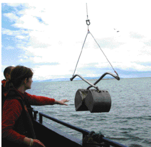
Fig 5.5 A grab for retrieving sea-bed samples. The variety and number of animal species present in the samples indicates benthic conditions. John Costelloe, Aquafact International Services.
