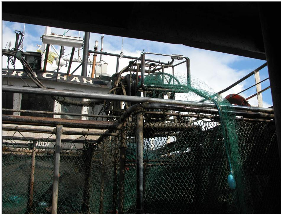
Figure 5. Net flaking machine and net pounds on MFV Berachah.
