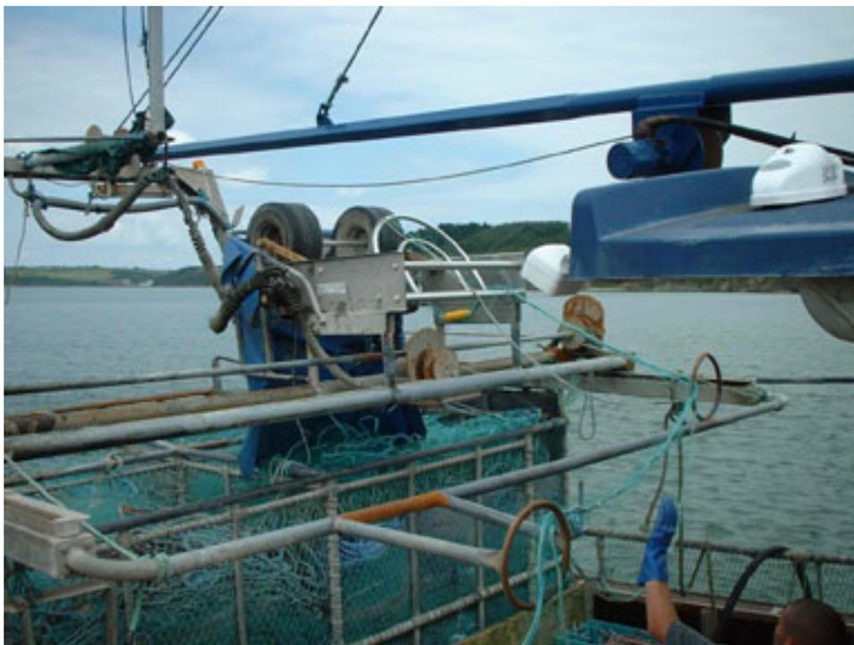
Figure 7. Net flaking machine and net pounds onboard MFV Western Dawn
