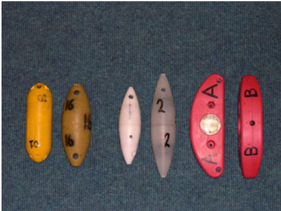
Figure 8. Airmar, Aquamark 100, Fumunda, Prototype Fumunda and Savewave (side and top view) pingers
